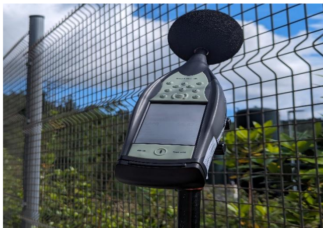
Typical noise monitoring
